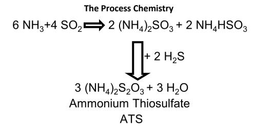
Sour gas path through the SimpliSWAATS unit travels through two successive contactors, scrubbing  $H_2S$  from sour gas by reaction with sulfite to produce ATS  $(NH_4)_2S_2O_3$ . The upper section of the process uses the required makeup water to wash sweetened gas to scavenge  $NH_3$ ,  $SO_2$ ,  $H_2S$ .
